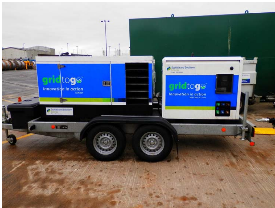
Figure 4 Bidirectional Hybrid Generation Plant
